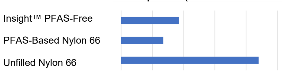
Figure 2 – Coefficient of Friction Comparison (Lower is Better)
