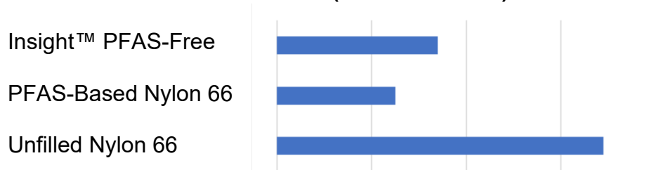
Figure 1 – Relative Wear Resistance (Lower is Better)
